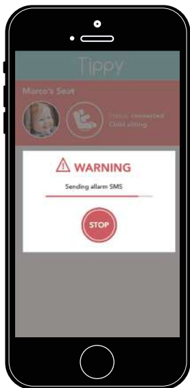
Picture 9. Alarm screen. For both Android and iOS platforms, the generation of alert SMS and alarm sound are triggered even if the application is in background state.
