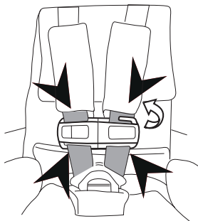
Figure 2. How to remove the chest clip that was supplied with the car seat.
