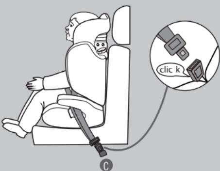
Lock the belt into the vehicle seatbelt buckle ensuring it clicks into place. Both the lap belt and the shoulder belt should pass through the belt guide on the side nearest the buckle (C).
