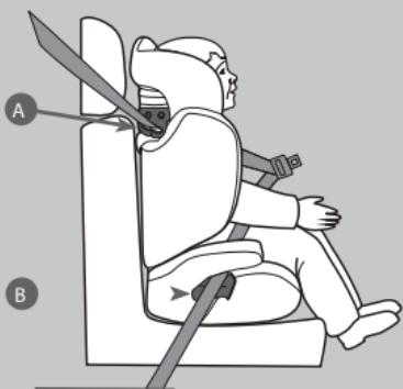
Put the child in the child car seat and adjust the size and fit of the seat (see previous step) then pass the vehicle's shoulder belt through the belt hook (A) and the lap belt through the lap belt guide (B).
