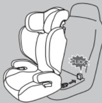
Rotate the bracket with ISOFIX anchors as indicated in the figure.
