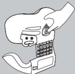
To adjust the height, width and fit of the child car seat, squeeze the adjust lever behind the headrest and move the headrest up or down until the desired height and width is achieved. Once the desired fit is found, release the lever and check the headrest to ensure it is locked and clicks into position.
