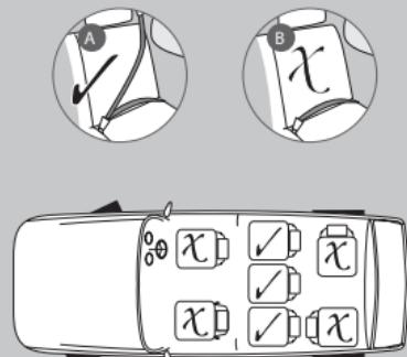
The car seat can be used only with 3 point seat belts (A) with ISOFIX anchorage point. DO NOT use it with 2 point seat belts (B).
