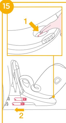
! To extend the ISOFIX connectors, press in and hold the ISOFIX adjustment button first. 15
