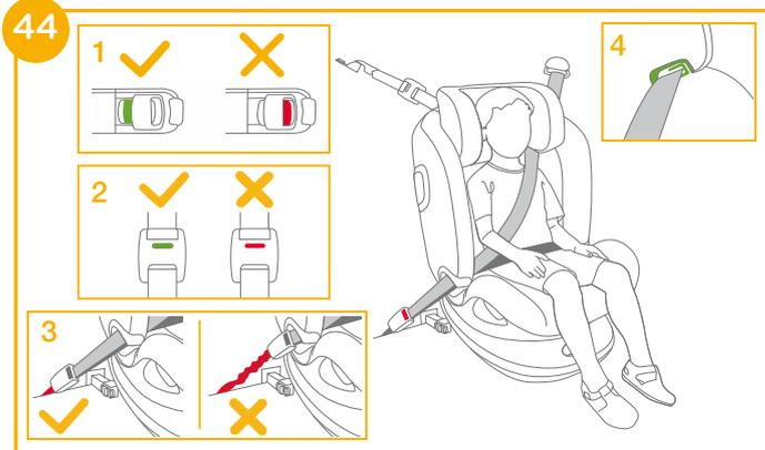
! The colors of the indicators on both ISOFIX attachments connectors should be completely green. 44-1
