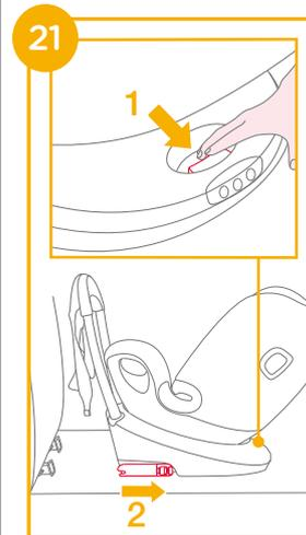
To extend top tether for use, press the button on tether adjuster and pull to lengthen. 22
