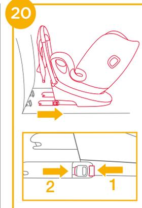
To prevent damage during transit, press the ISOFIX adjuster button 21 -1 and fold the connector completely. 21 -2
