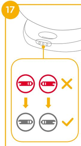
! Press the ISOFIX adjustment buttons again while pushing the seat back until it comes in contact with the vehicle seat backrest. 18
