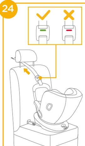
! If recline angle is adjusted, check the tension on the top tether, or loosen to adjust angle then re-tension. 25
