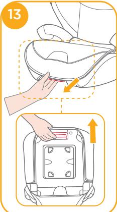
Rotate the ISOFIX connectors 180 degrees until they are pointing in the direction of the ISOFIX guides.
