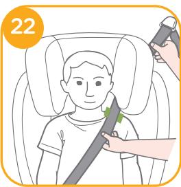
! Make sure, that the shoulder belt portion of the vehicle belt goes straight through the shoulder belt guide as shown in 23
