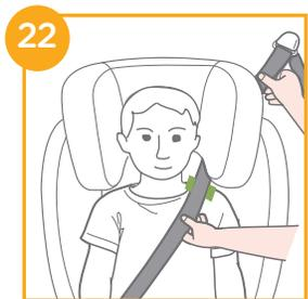
! Make sure, that the shoulder belt portion of the vehicle belt goes straight through the shoulder belt guide as shown in 23
