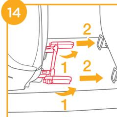
3. Line up the ISOFIX connectors with the ISOFIX anchor points, and then click both ISOFIX connectors into the ISOFIX guides. <sup>15</sup>
